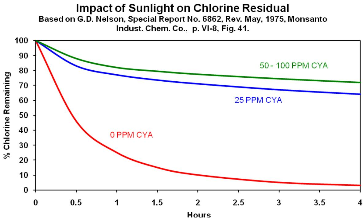
When cyanuric acid is used, hypochlorous acid is always in equilibrium with cyanuric acid-bound available chlorine. As suggested by the equation below, the stabilization of chlorine residual results from a reaction of free chlorine (hypochlorous acid or hypochlorite) with cyanuric acid to give cyanuric acid-bound available chlorine.
